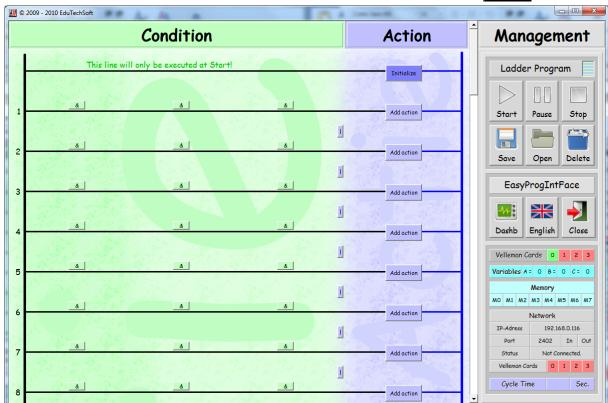
If one or more Velleman cards are connected (K8055 or VM110), the connected cards should appear green in the window right at the right hand bottom of the screen.
